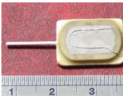
Figure 2 Photograph of the sensor after 8000 hours tests.
