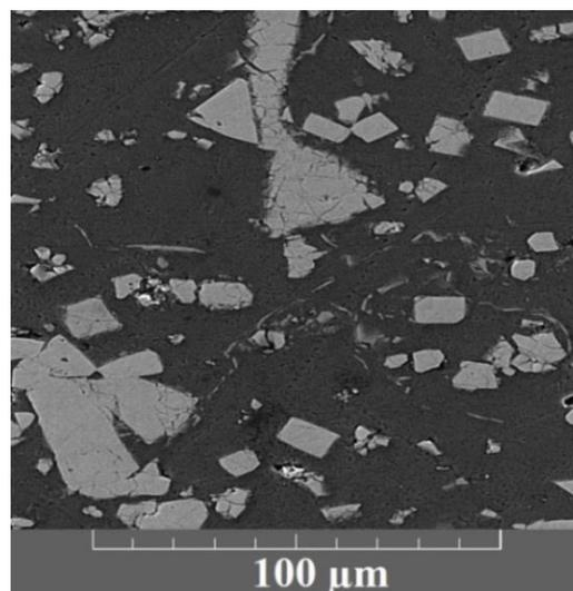
**Figure 2** Microphotograph of Al-Zr alloy containing 10 wt. % Zr.
