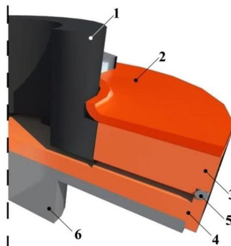
**Figure 1** Scheme of the rapid quenching installation: 1 – graphite supercharger; 2 – pressure disk; 3 – upper cooling disk; 4 – lower cooling disk; 5 – external sealing ring; 6 – electric motor flange.
