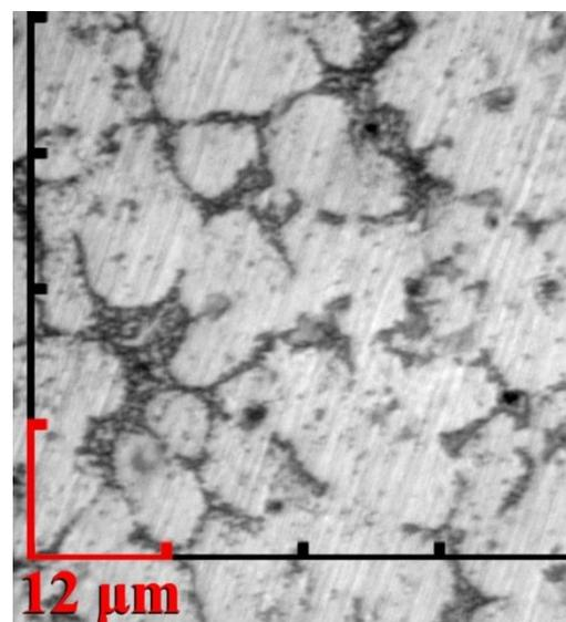
**Figure 8** Microphotograph of the AK6 alloy with a Zr content of 0.5 wt. %, obtained at a cooling rate of  $10^3$  K/s.**Table 3** – Properties of AK6 alloys with different zirconium contents after quenching.
