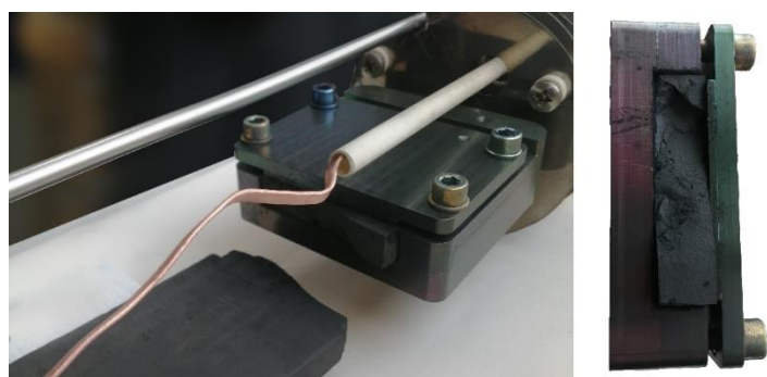
Figure 2 Ceramic anode failure that occurred during thermal testing in an experimental cell with a current of 50 A.
