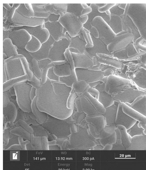
Figure 1 Refinement of the XRD for the composition \text{Ba}_{0.9}\text{Ca}_{0.1}\text{LaInO}_4 . Figure 2 SEM image of the \text{Ba}_{0.9}\text{Ca}_{0.1}\text{LaInO}_4 ceramic sample.
